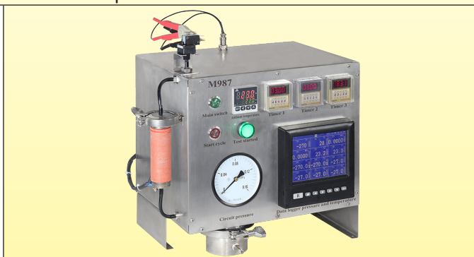
Test equipment for measuring, recording and setting the barometric and the ambient temperature compensation systems of the air switches (Ultimheat Laboratory)
